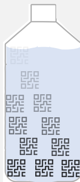
Figure 8. Illustration of watermark technology where camera sees QR-codes, but consumers see a regular water bottle. (Own illustration, modified from AIM, n.d.)
