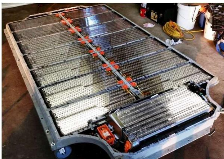
Figure 15: 2017 Tesla Model S battery pack. The battery pack as 16 modules, and 7104 cells. (Cuma, 2017)
