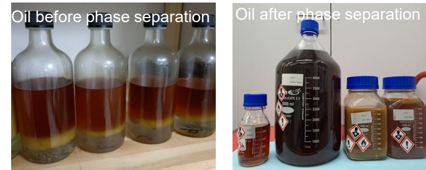
Fig 2: Feedstock received for catalytic hydrotreatment
